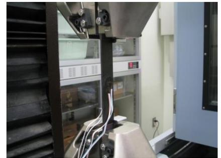
ASTM D3039(無孔引張試験)
